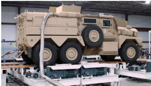
Military MRAP Multi-function End-of-Line test stand
