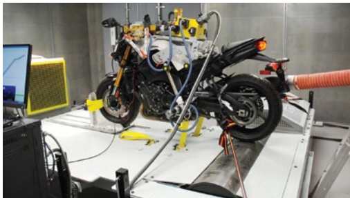
Self-contained end-of-line test cell including robotic actuators for self-driving
