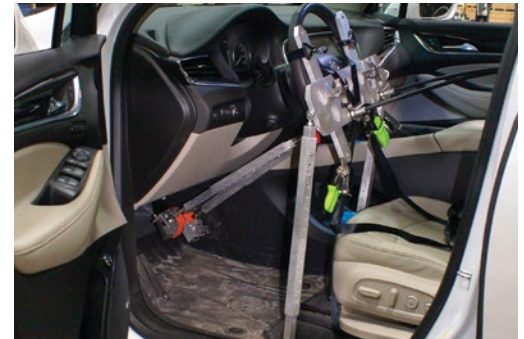
Robotic pedal-throttle actuators for automatic driving
