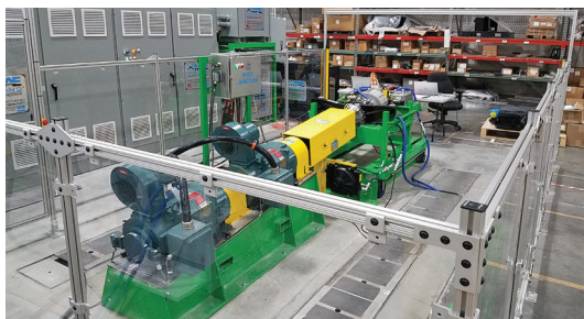
EV drivetrain test cell
