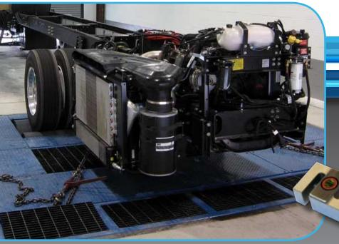
Mustang's Vehicle Simulation capabilities are made possible by using powerful eddy current power absorbers and torque sensing load cells that provide an ultra-fast closed loop signal to the dyne controller. Mustang's dynamometer control technology is recognized around the world as the industry's best.
