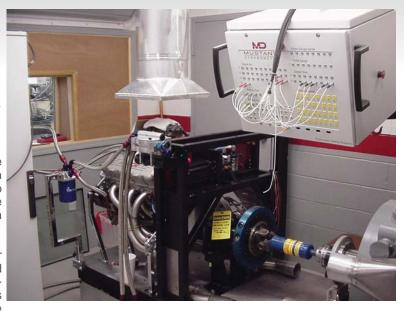
1200-hp Electric AC Dynamometer with a Rockwell Automation Regenerative Drive has been selected as the dynamometer for the MD-AC-1200-10K primarily due to its superior response, load control accuracy, load stability, transient features, and full speed range capabilities (0-10,000 RPM). Through regeneration, the majority of the power absorbed by the dynamometer is returned to the user's power grid - resulting in a substantial reduction in operating costs associated with the test stand.
