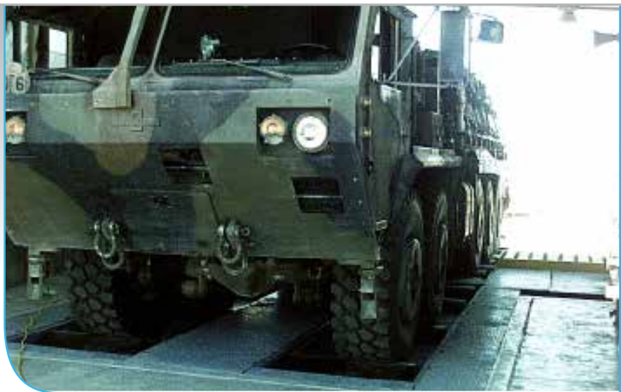
Multi-Axle Chassis Dynamometer in Extreme Climatic Test Chamber.
