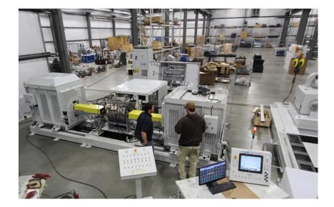
The test stand's power absorption units are bi-directional eddy-current PAUs which provide high performance loading torque. The PAU's are capable of up to 2,000 lb-ft of dynamic load torque with a maximum speed of 4,000 rpm. Air actuated caliper brakes are incorporated into the load units for stall testing.
