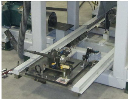
FIGURE 2 - TAIL ROTOR GEARBOX BEING LOADED INTO TEST STAND
