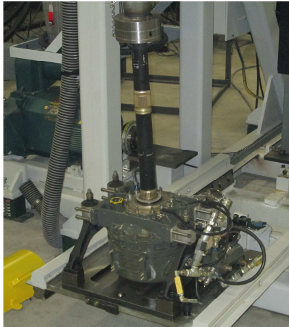
FIGURE 1 - MAIN GEARBOX BEING LOADED INTO TEST STAND
