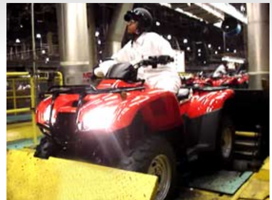
The multi-function tester in action testing Honda ATVs as they come off the line at Honda South Carolina's Timmonsville ATV Assembly Plant.
