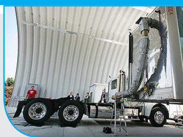
48" (1,219mm) Dual Axle AC Dyne at Univ. of California Riverside Emissions Lab
