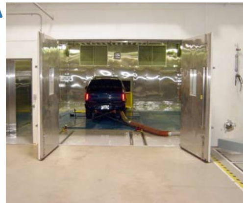
Photo of upgraded test cell with newly installed AWD 48" AC Motor Chassis Dynamometer by Mustang Advanced Engineering.
