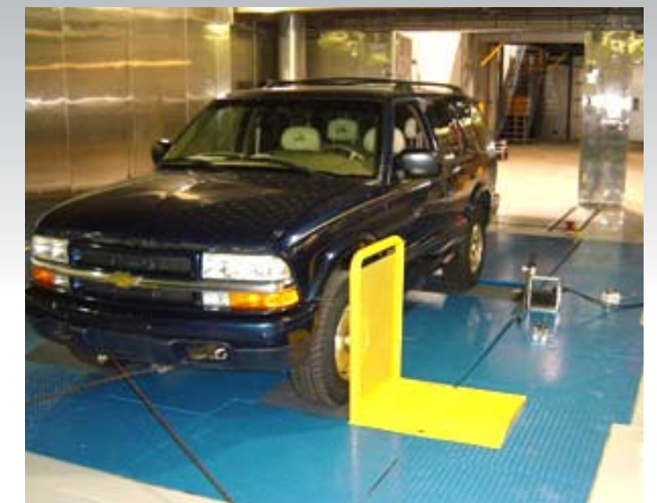
↑ New dyne in test cell showing remote pedal controller outside of vehicle at the moment.
