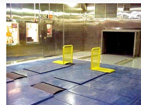
← New dyne in test cell showing wind tunnel nasal and control room windows.
