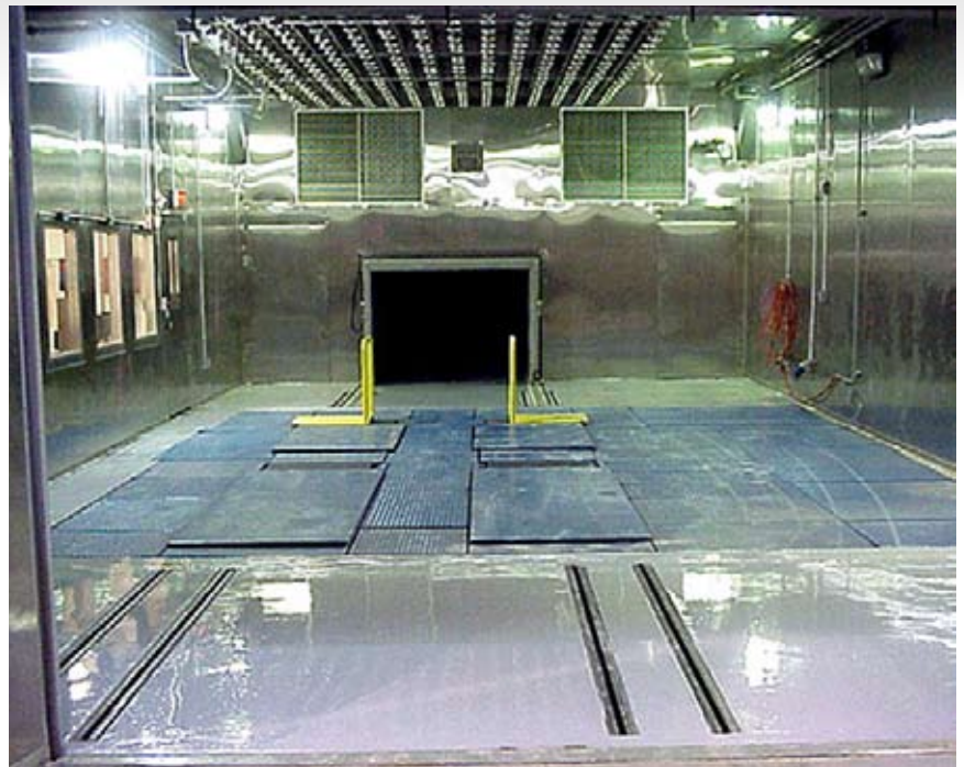
Photo of upgraded test cell with newly installed AWD 48" AC Motor Chassis Dynamometer by Mustang Advanced Engineering.
