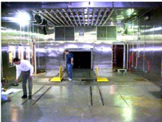
Photo of existing test cell with 2WD eddy current chassis dynamometer prior to start of test cell upgrade.
