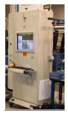
The Cab Test System must consist of a Pentium-based Desktop or Industrial Computer, mobile NEMA 12/13 Fan-Cooled Enclosure, 24" LCD Color Monitor, NATIONAL INSTRUMENTS Data Acquisition Hardware, 1500/1800 BTU Air Conditioning Unit, DC power supplies, Active Load Resistors, Fast-Acting Circuit Breakers, RF Radio Remote Control, wired Barcode Scanner, one (1) custom Test Harness, and custom application test software.
