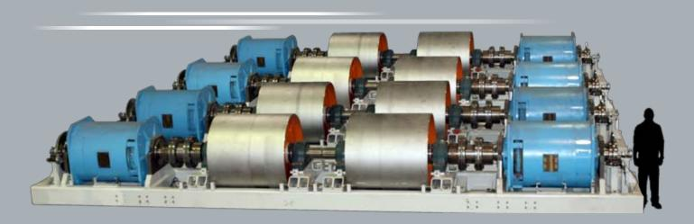
Tests that the system can perform include, but are not limited to hybrid calibration, dynamic performance test, fuel economy performance test, ABS braking performance test, emissions performance test, creeper gear performance test, constant speed, constant force, constant torque, constant power, controlled acceleration and vehicle simulation road load testing.
