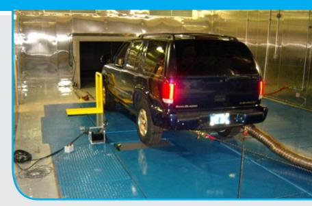
AWD 48" Chassis Dynamometer in Thermal, Climatic & Solar Wind Tunnel
