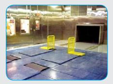
AWD 48" Chassis Dynamometer in thermal climatic and wind test chamber showing wind tunnel nosal and dyne control room windows.
