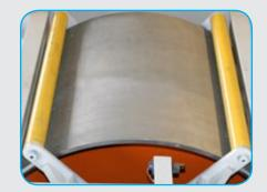
A pair of vehicle centering guards aid in positioning the wheels on the rollers and can also raise the vehicle for free coast down of the system.
