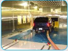
AWD 48" Chassis Dynamometer showing an optional vehicle restraint system and exhaust removal system.
