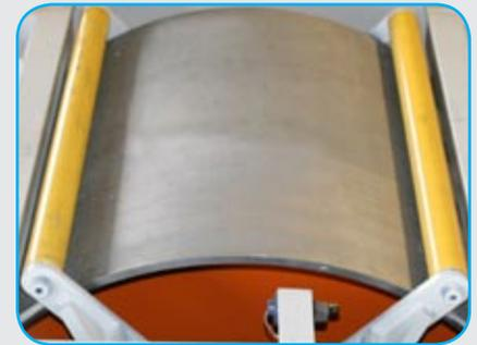
A pair of vehicle centering guards aid in positioning the wheels on the rollers and can also raise the vehicle for free coast down of the system.
