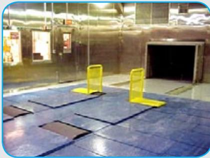
AWD 48" Chassis Dynamometer in thermal climatic and wind test chamber showing wind tunnel nasal and dyne control room windows.
