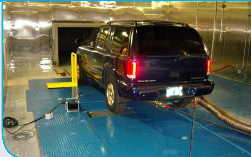
AWD 48" Chassis Dynamometer in Thermal, Climatic & Solar Wind Tunnel
